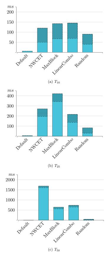
Figure 4.12: Execution time of "Taking-One-Partitioning" approach (in ms)
