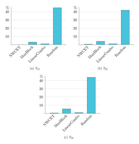
Figure 4.11: Percentual error of "Taking-One-Partitioning" approach
