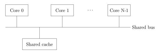
Figure 1.3: Concept of a multi-core system
